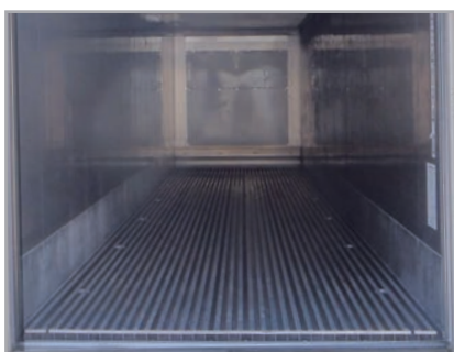
Container interior : T floor and walls
